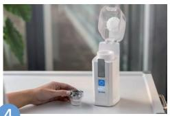
After grinding, open the lid and take out the SeveroCup together with the grinding head. Check the cup for visual contaminations. Remove the grinding head while keeping the SeveroRondel in the cup.
